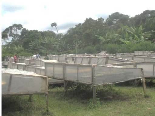
Figure 1. Direct Solar Dryer models used for drying pineapple slices in Kayunga
