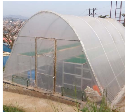
Figure 2. Tunnel solar dryer at Makerere University
